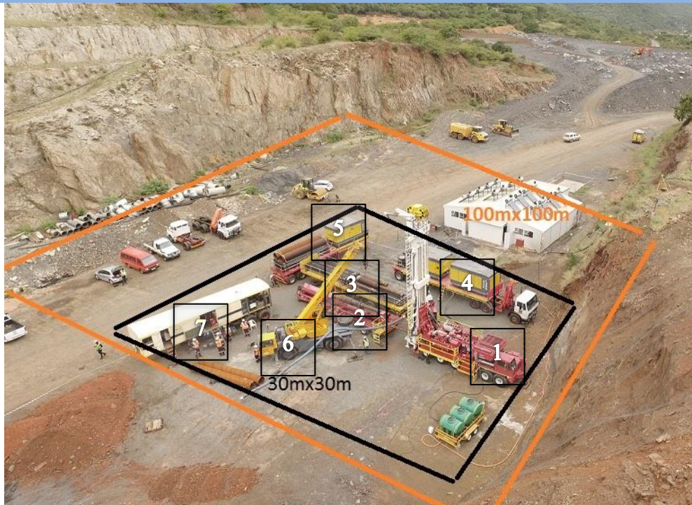
Figure 1: Typical arrangement of vehicles when RDU is deployed.
